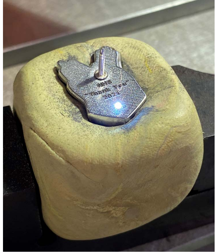
At our finishers in Birmingham the sprue is removed, the hands fettled and polished and pin attached to the back. The very last procedure to be done is to laser engrave the text on the back, NHS "Thank You" 2021.
