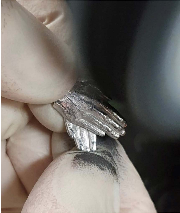
At our finishers in Birmingham the sprue is removed, the hands fettled and polished and pin attached to the back. The very last procedure to be done is to laser engrave the text on the back, NHS "Thank You" 2021.
