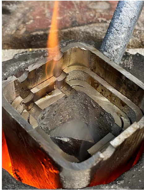
A section of 1939 vintage Spitfire main spar is heated until it becomes molten at around 700 degrees centigrade. Once liquid the hot metal is poured into the previously made casting flask.
