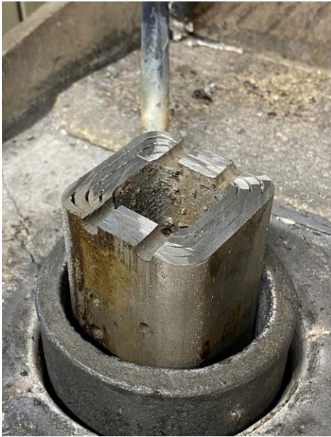
A section of 1939 vintage Spitfire main spar is heated until it becomes molten at around 700 degrees centigrade. Once liquid the hot metal is poured into the previously made casting flask.
